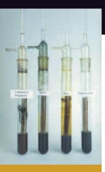
This is a simulation of what a compressor lubricant is subjected to in a severe application. Other synthetic fluids show varnish and deposit formation, leaving Ultra Coolant the clear winner.
