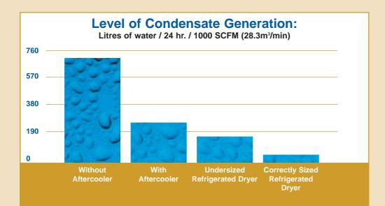
A 75 kW compressor operating with an aftercooler for 8,000 hours a year will produce over 38,000 litres of condensate, enough to fill a swimming pool. The good news is most waste water regulators accept direct discharge of condensate from compressors running with Ultra Coolant.
